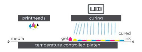
The UVgel process results in high-quality print output thanks to optimal dot gain control at productive speeds. prints can be finished with a matte of glossy look without changing the ink or the media. UVgel prints are very robust; lamination is not always required. If to be laminated, lamination can happen immediately thanks to instant dry prints.
